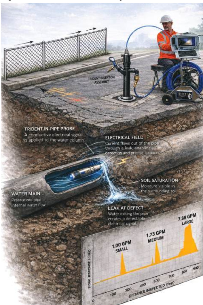
Figure 33. Electro Scan's Field Set-Up.
