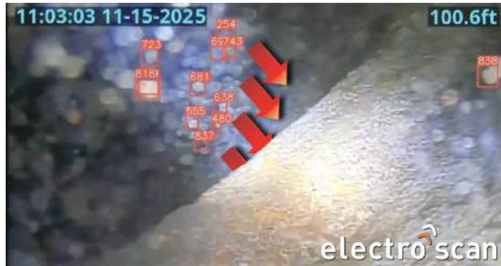
Figure 32. Electro Scan's AI-CCTV Particle Tracing.
