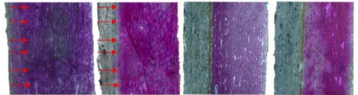
Asbestos Cement Pipe Pipe Wall Thickness Measurement
