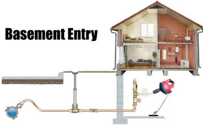
Figure 26. A Typical Basement Entry for SWORDFISH Survey.
