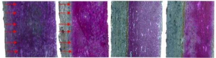
Asbestos Cement Pipe Pipe Wall Thickness Measurement
