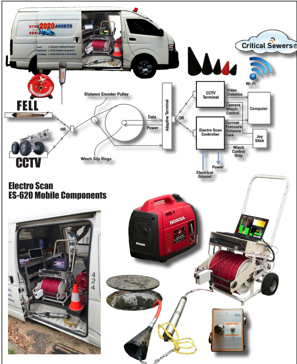
Figure 16. Field Set-Up Configuration for Sydney Water Electro Scan Trial
