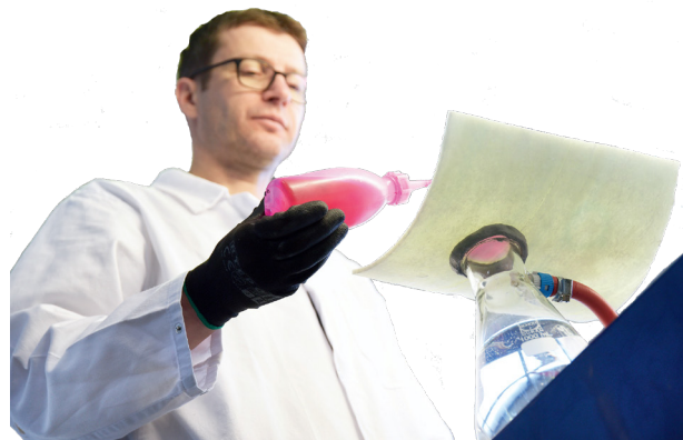
Figure 10: Cured-In-Place Pipe Lining Test by IKT
