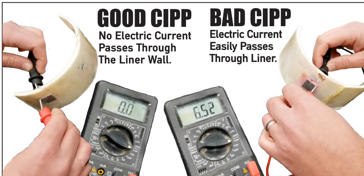
Figure 9: CIPP Lining Evaluated With Electric Current
