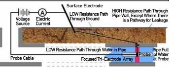
ASTM F2550-13 standard covers the location & measurement of all cracks, fissures, broken joints, and leaking service connections, by measuring the change in electrical current able to pass through defects in a pipe wall.
