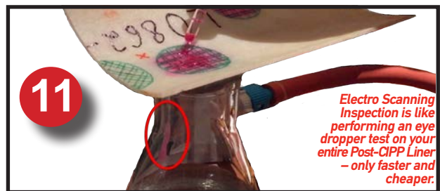
11. Defective/ Porous/ Weak Liner
