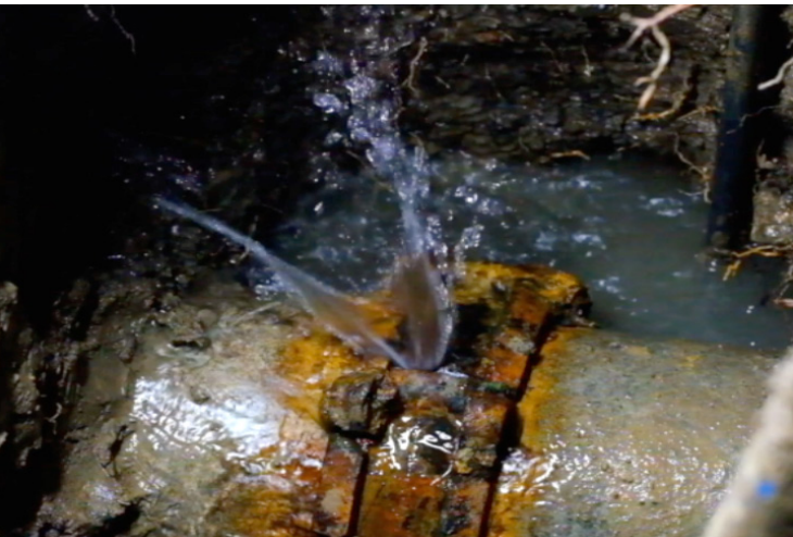
Low voltage conductivity finding defects missed by legacy inspection techniques.
