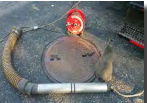
(Above) ES-620 for Sewer Mains, Grounding Reel, and Sliding Funnel Plug.
