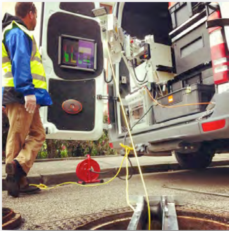
Figure 16. Data automatically displayed on Operator's Real Time Console, requiring no data entry or interpretation during scanning process.
