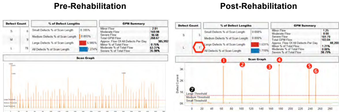
Figure 24. Sample Pre-Rehabilitation and Post-Rehabilitation, i.e. before and after, condition assessment reporting.
