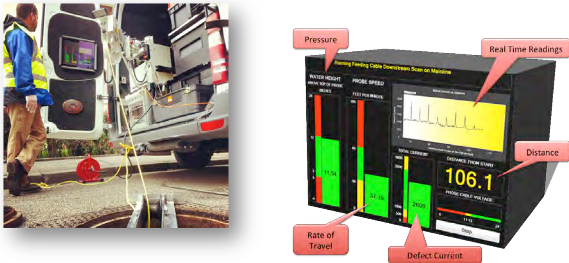
Figure 16. Data automatically displayed on Operator's Real Time Console, requiring no data entry or interpretation during scanning process.
