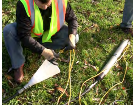
Field Tech, Macy Grubbs, attaches a Funnel Cone to Jet Hose and Electro Scan Probe.
