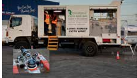
(Left) Specialty equipment designed and developed for Rangedale to inspect large sewer interceptors for Melbourne Water. UVS operates is the leading CCTV camera repair facilities in Victoria.
