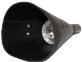
(Above). Electro Scan's funnel plug, attaches to a jet hose from the downstream manhole to create a reservoir of water surrounding the ES-620 probe. The Electro Scan Funnel Plug, available for all diameters of 6" to 20" allows water to surcharge around the probe, preventing the need to fill an entire sewer main. If the sewer pipe is already filled, there is no need to use the funnel plug.
