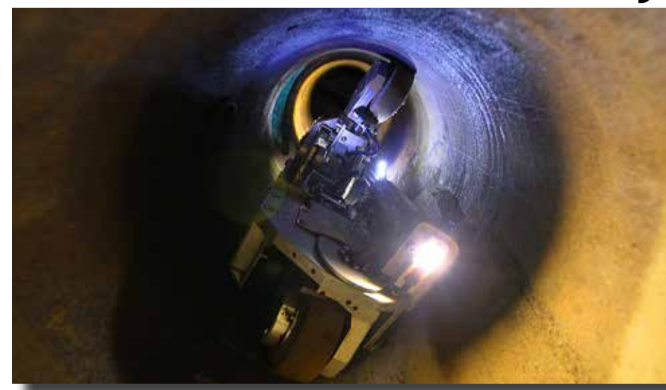
Pictured above: CISBOT, the cast iron joint sealing robot, from ULC Robotics internally sealing leaking joints inside a cast iron gas main
