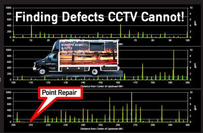
(Above) A sewer agency used CCTV to locate a defect that was determined to require a Point Repair at 210 feet. A Point Repair was completed and the Contractor used CCTV to certify the repair. Then, the pipe was Electro Scanned.
