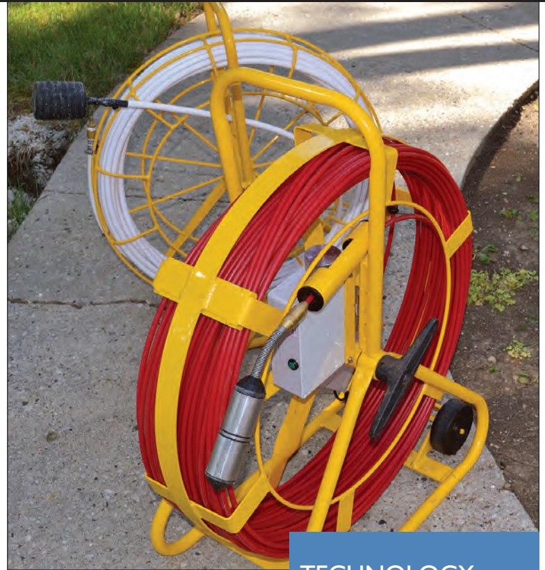
The Electro Scan ES-38 probe, attached to its cable and ready for use. The reel of white hose behind it carries the inflatable sewer line plug used to block the line during the test. (Photography by Matt Gunn)
