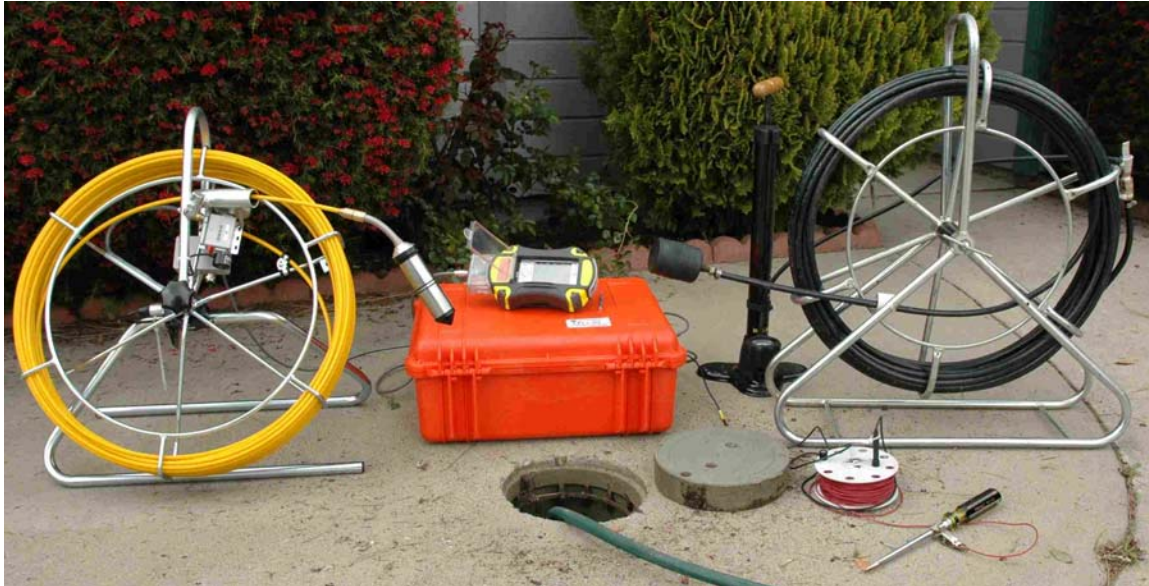
Figure 3. FELL-21 System Equipment
