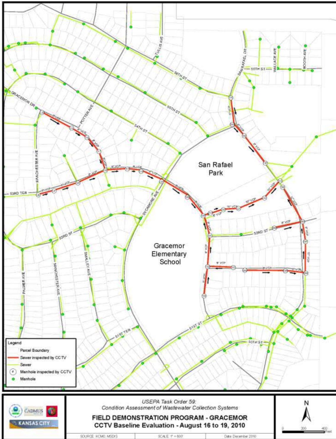
Figure 4-1. Pipe Segments Inspected by CCTV in the Gracemor Area.
