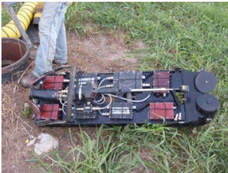
Figure 4-14. Float Set on Ground after Completion of Sewer Inspection Work.
