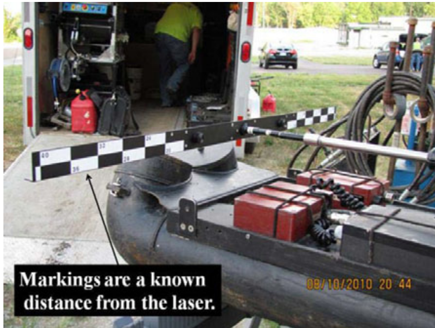
Figure 4-12. Calibration Device for the Laser.
