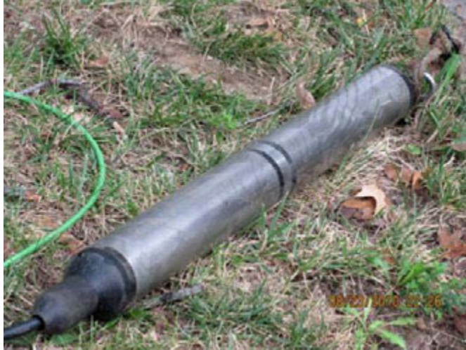
Figure 3-3. Sonde for Electro-scanning Unit.
