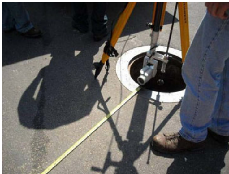
Figure 4-5. Calibration of Zoom Camera to Measure Distance.
