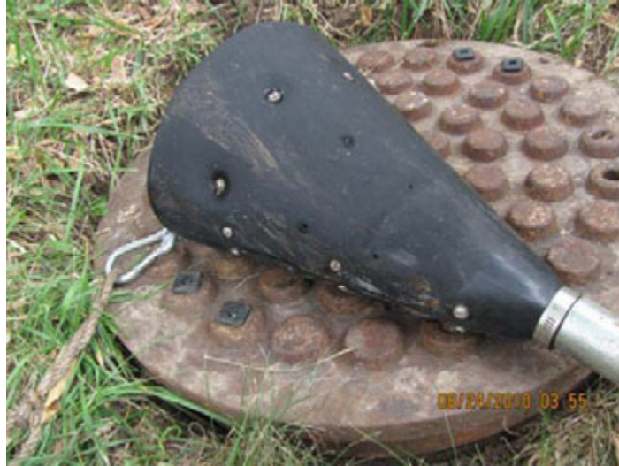
Figure 3-4. Sliding Plug for Electro-scanning Equipment.
