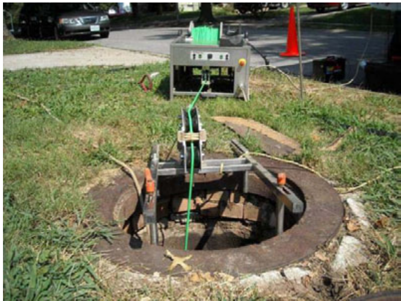
Figure 3-7. Cable and Cable Guides for Electro-scanning Inspection.
