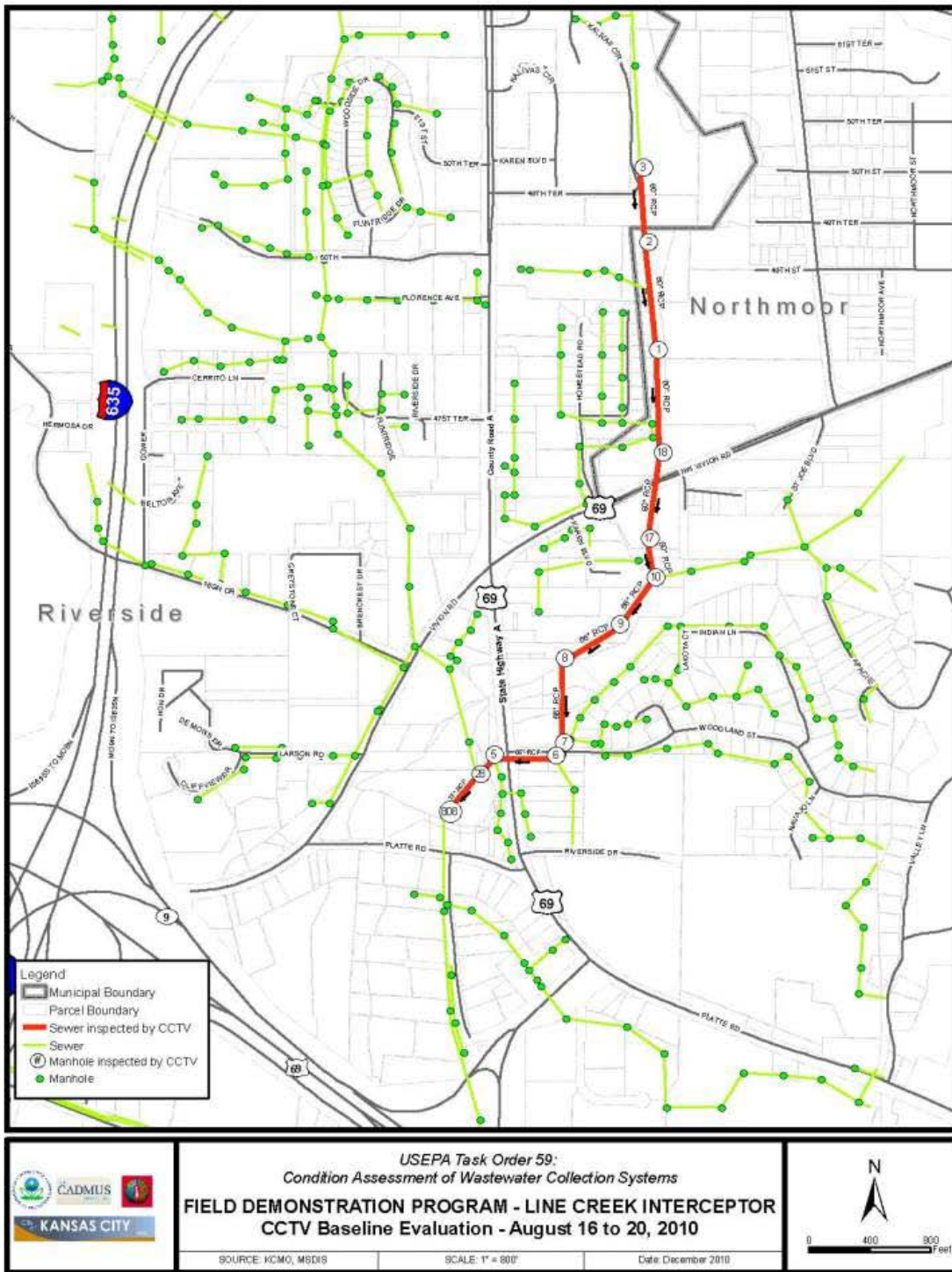
Figure 4-2. Pipe Segments Inspected by CCTV in the Line Creek Interceptor.
