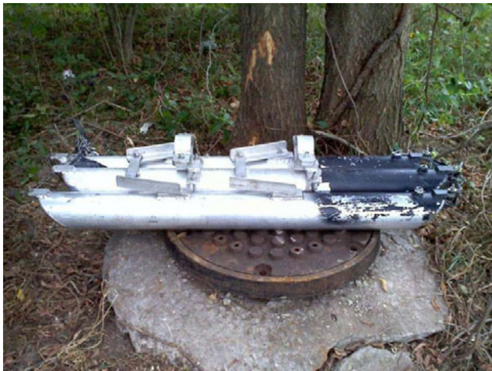
Figure 3-1. Custom Pontoon for Floating CCTV Camera in Large-Diameter Sewer.
