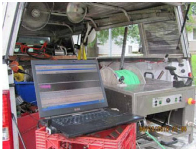
Figure 3-9. Inspection Truck with Laptop and Cable Spool/Winch.
