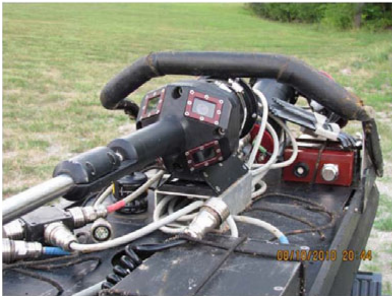
Figure 3-11. Fly-Eye Array of Four Cameras for Laser Profiling Imaging.
