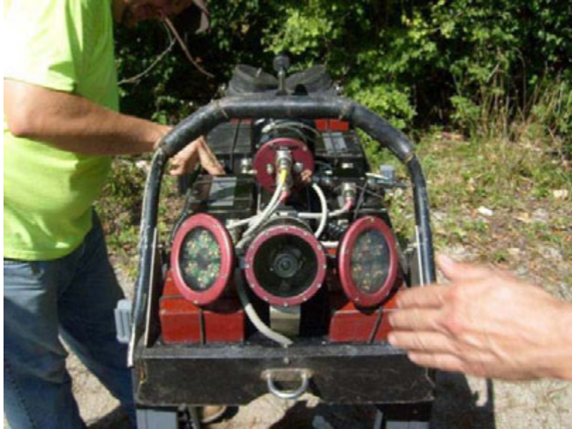
Figure 3-10. HD Camera and Twin LED Lights at Front of Float.
