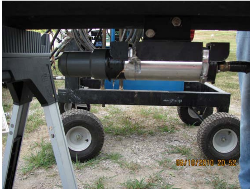
Figure 3-12. Sonar Head on Multi-sensor Float Assembly.
